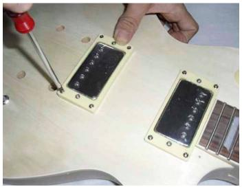
Secure the frames with dome-head screws into the pre-drilled holes.
