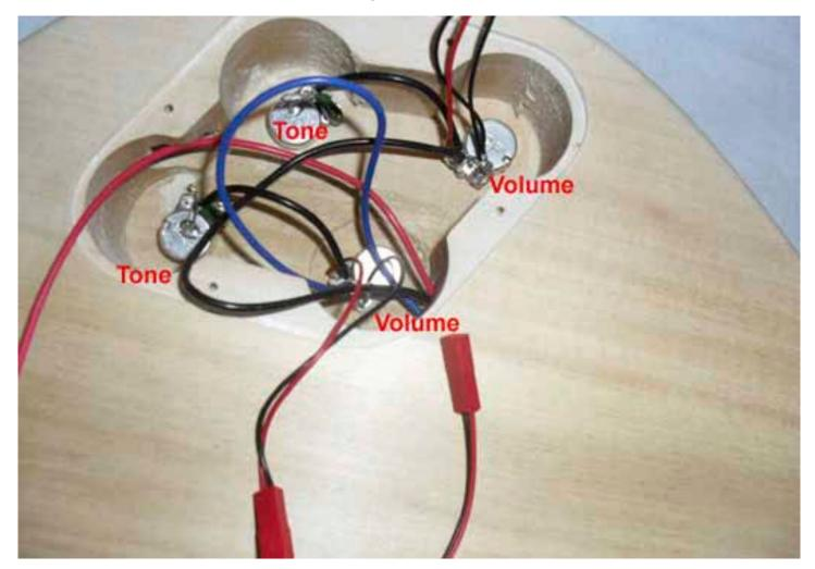
Take out the cable without connector (string grounding cable) and insert it into the pre-drilled bridge hole through the channel. Just leave it in the bridge hole. It will connect to earth when the boots of the bridge are pressed on it. String grounding reduces noise (hum).
